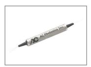
ACP's 1480/1550 WDM/Isolator Hybrid component utilizes thin film coating technology and and proprietary designed metal bonding micro optics packaging to achieve optical signal and pump power combining and back reflection signal elimination. It provides low insertion loss, high isolation, wide pass band, low temperature sensitivity and epoxy free optical path. It can be used for EDFA application.
